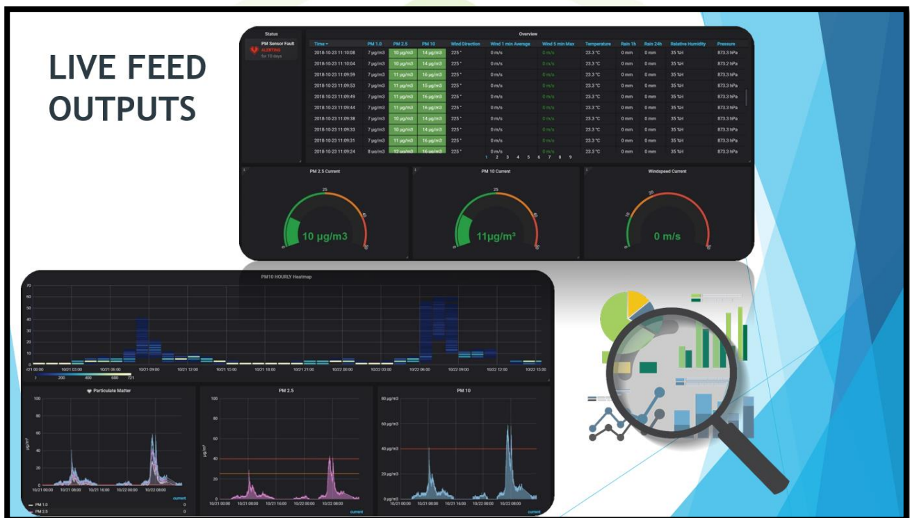
Figure 12: Typical Real-Time Ambient Particulate Matter monitoring dashboard communication interface
