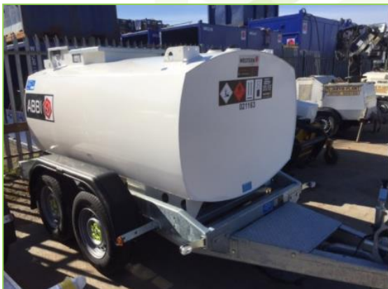
Figure 3.6: Typical mobile fuel storage trailer with bunded tray
