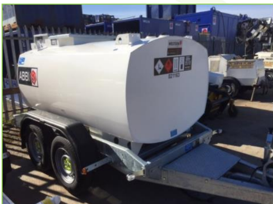
Figure 4-4: Typical mobile fuel storage trailer with bunded tray
