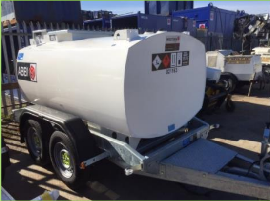
Figure 3-7: Typical mobile fuel storage trailer with bunded tray
