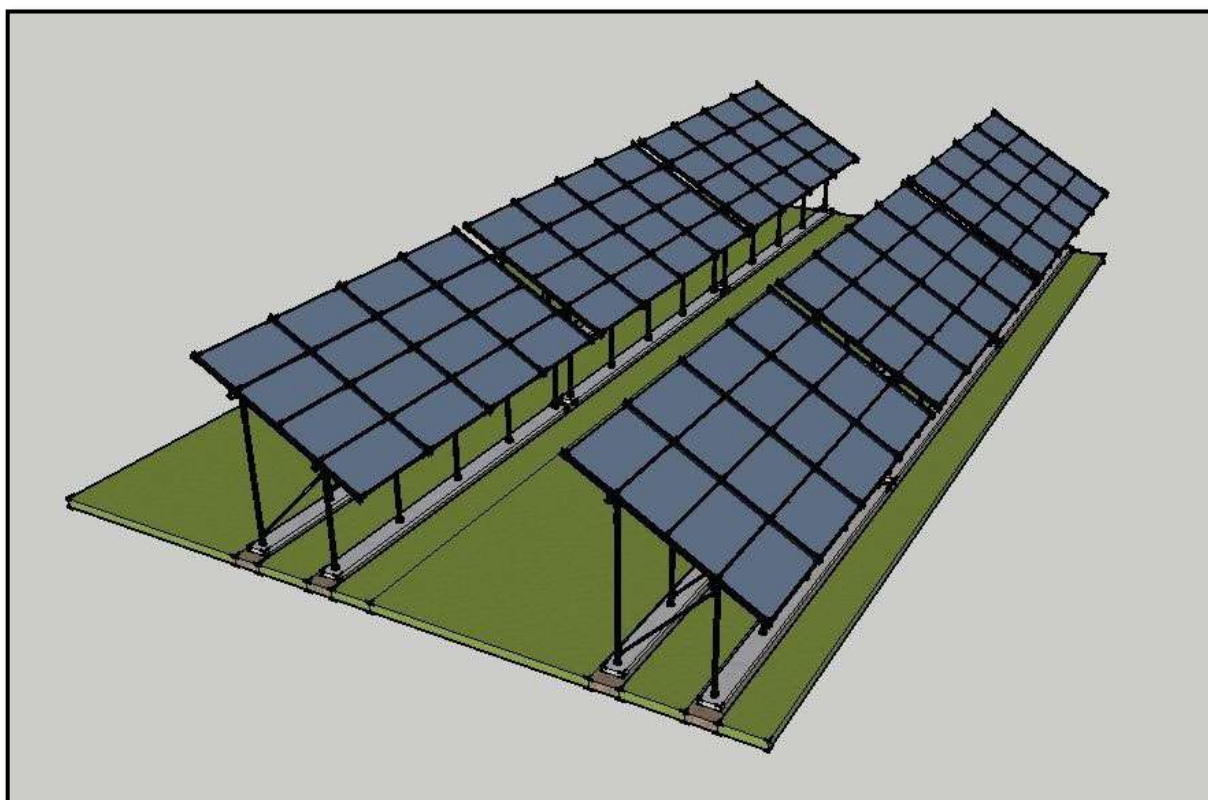
Figure 5.2.1: This Figure depicts a 3D image of a single array in a 1MW block.
