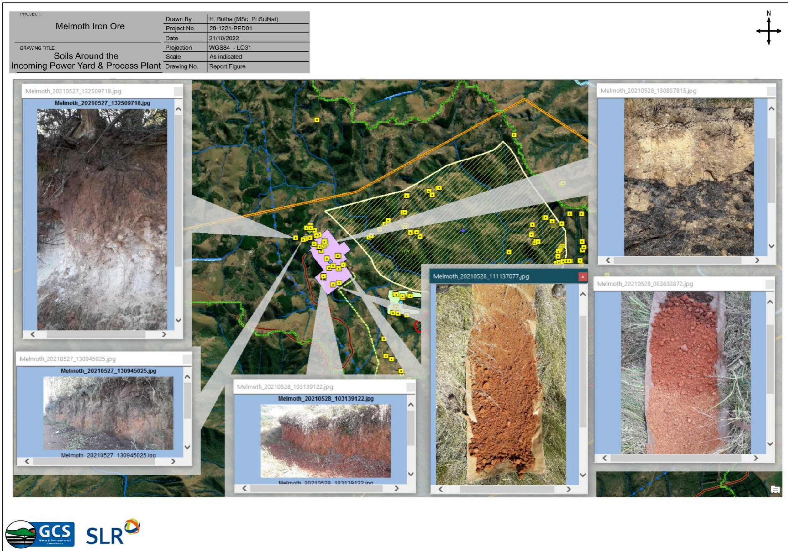
Figure 2-25: Soil observations - surrounding the proposed incoming power yard and processing plant
