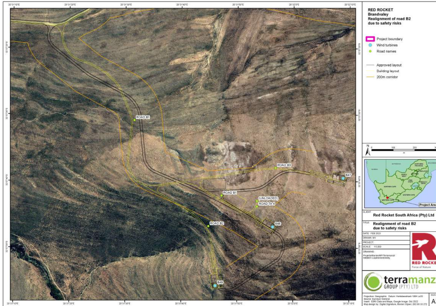
Figure 2.6: Map indicating the minor realignments of road B2 (in Yellow) in comparison to the previously approved and authorised layout (in Black) with the authorised 200m Corridor (in Orange)
