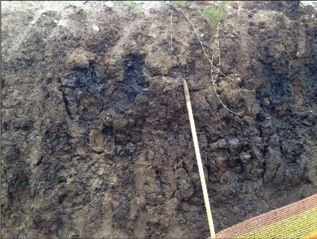
Plate 10. View of tar residue seeping out of pit wall on Tar Dam A (South)
