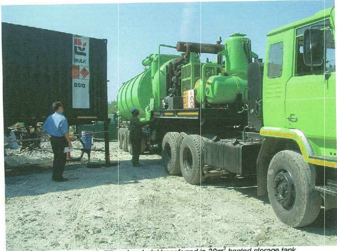
Photograph 15: Filtered material transferred to 30m 3 heated storage tank
