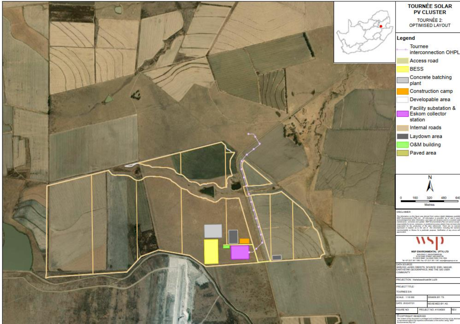
Figure 2-1 – Tournée 2 Solar PV Facility Final Layout
