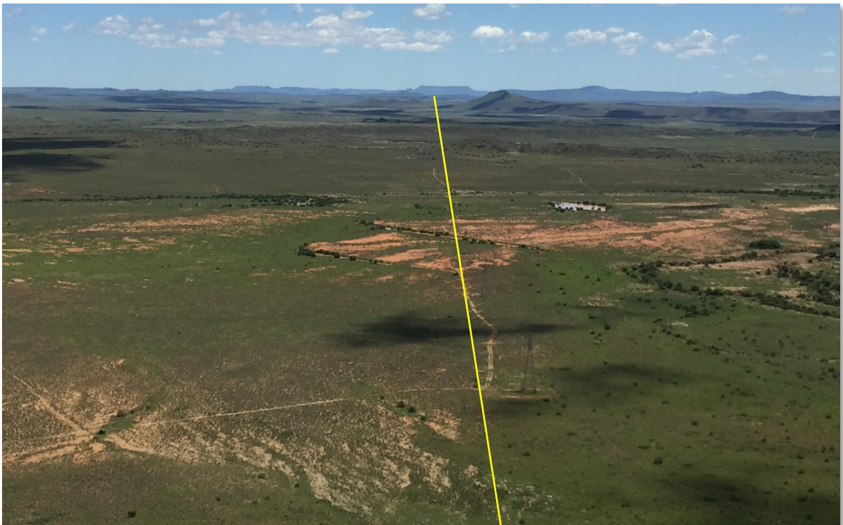
Plate 2:View from the plateau across the proposed alignment of grid connection Route 1. De Aar and the Hydra substation are located below the hills on the horizon. Note the open erosive areas in the foreground which are typical of the valley bottoms traversed by the route. The yellow line shows the approximate route of the new grid connection. The existing power line is visible to the right of the proposed route.
