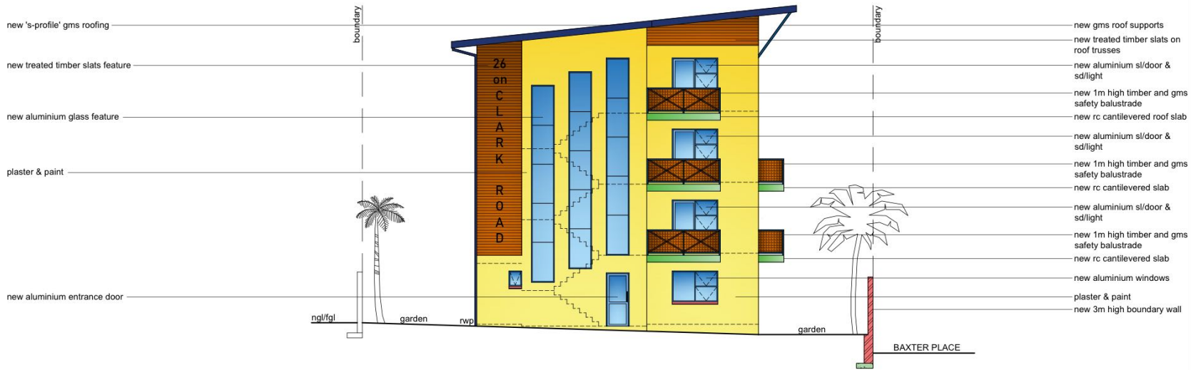
SOUTH WEST ELEVATION
