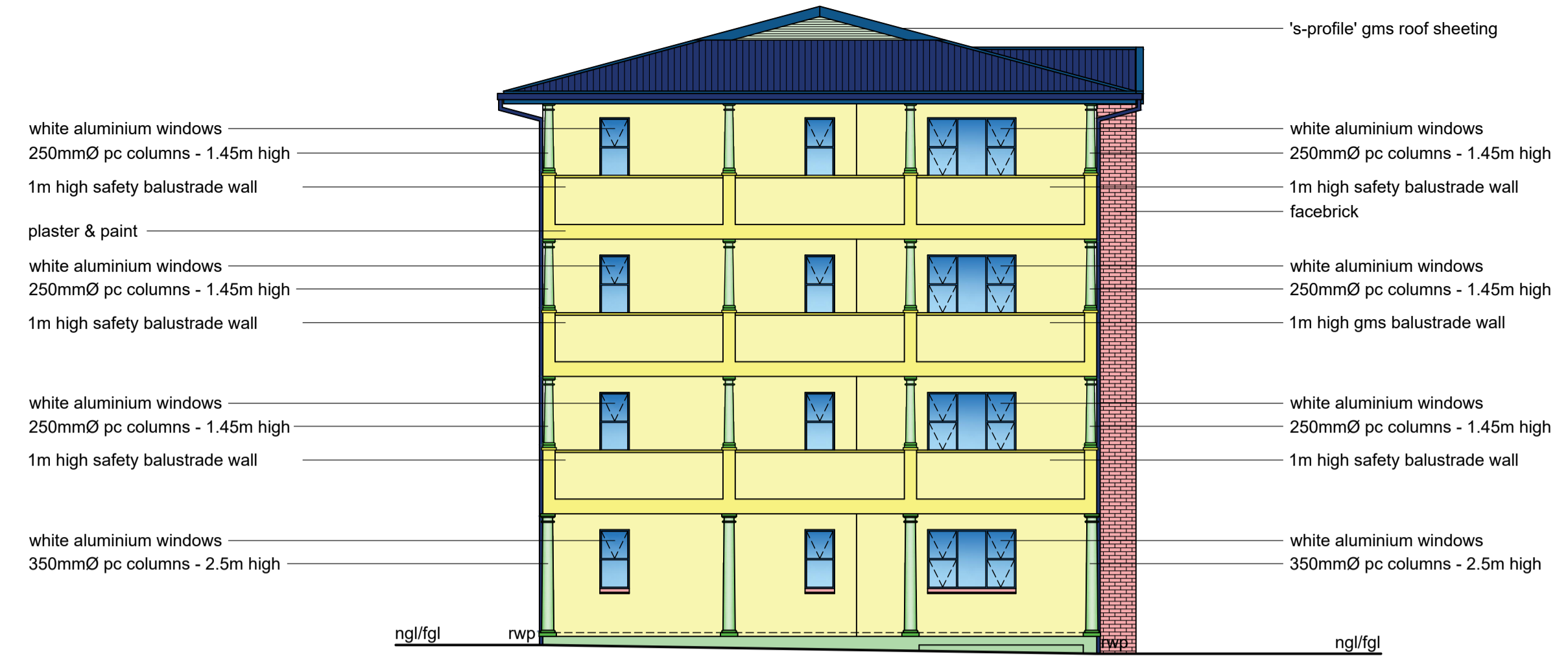
SOUTH WEST ELEVATION
