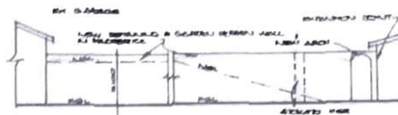
ELEVATION RETAINING WALL
