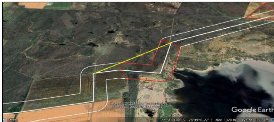
Figure 2 The yellow line depicts the proposed deviation in the 44 kV route to avoid an area of high collision risk (polygon depicted in red along the 300 m corridor)
