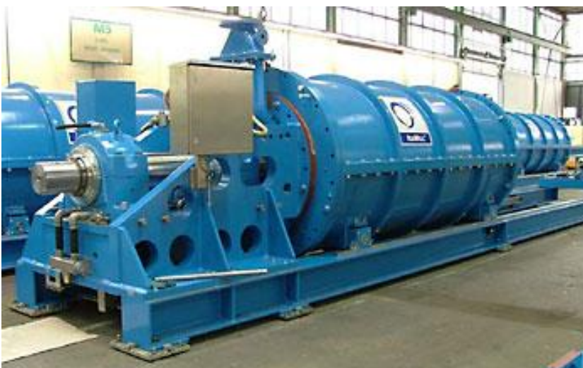
Figure 15: Example of an IsaMill™
