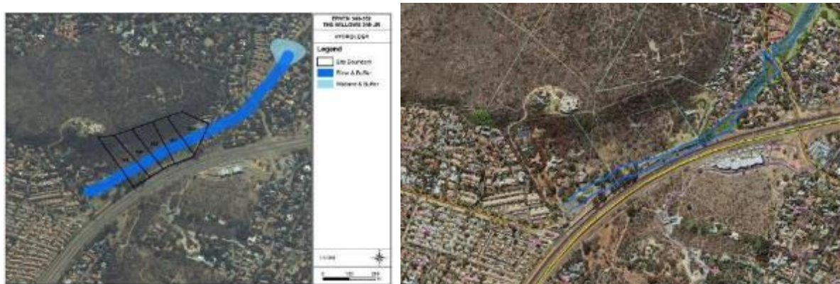
Figure 3.4: Left: A drainage line according to the GDARD website. Right: The flood lines of the drainage line (Supplied by Environment and Agriculture Management Department, City of Tshwane)
