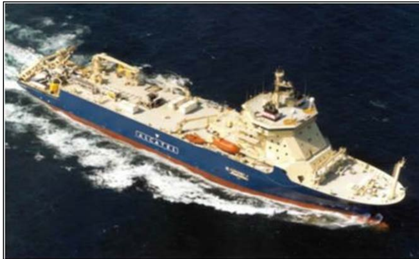
Figure 2 Typical Cable Laying Ship
