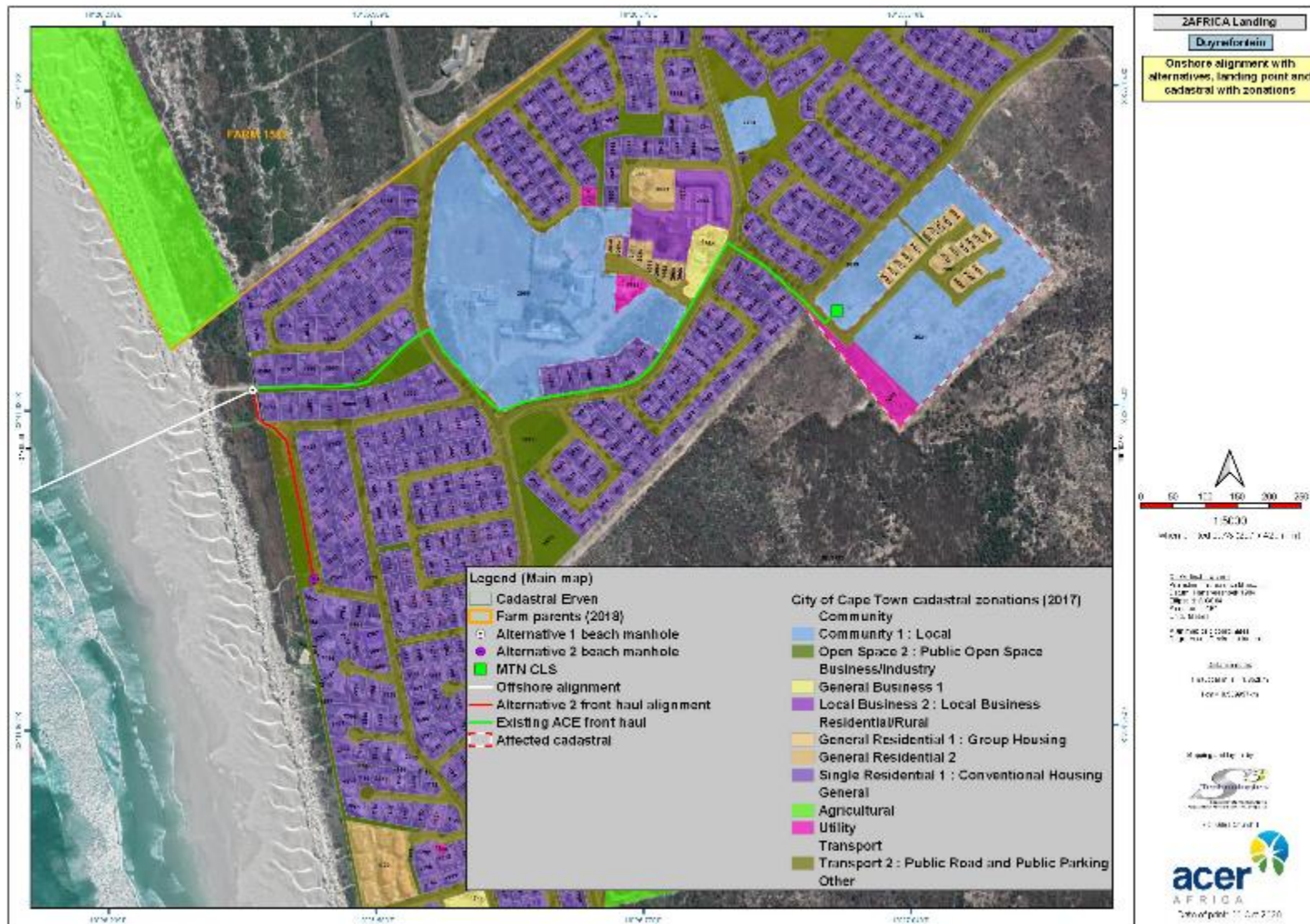
Figure 13 Proposed cable alignment from Alternative Landing Sites 1 and 2 to the MTN CLS site in Duynefontein
