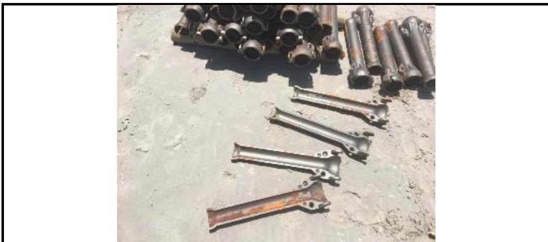
Plate 9 Articulated pipe sections which are installed around the cable in shallow water to offer additional protection.
