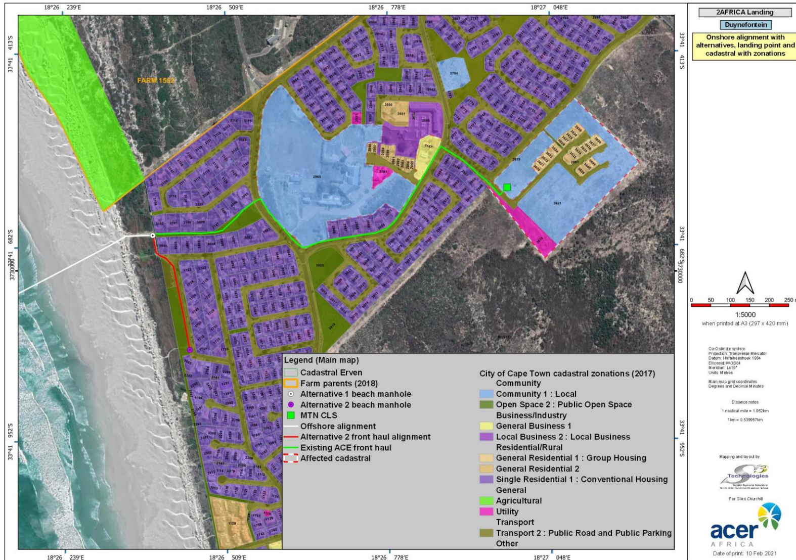
Figure 13 Proposed cable alignment from Alternative Landing Sites 1 and 2 to the MTN CLS site in Dufnefontein
