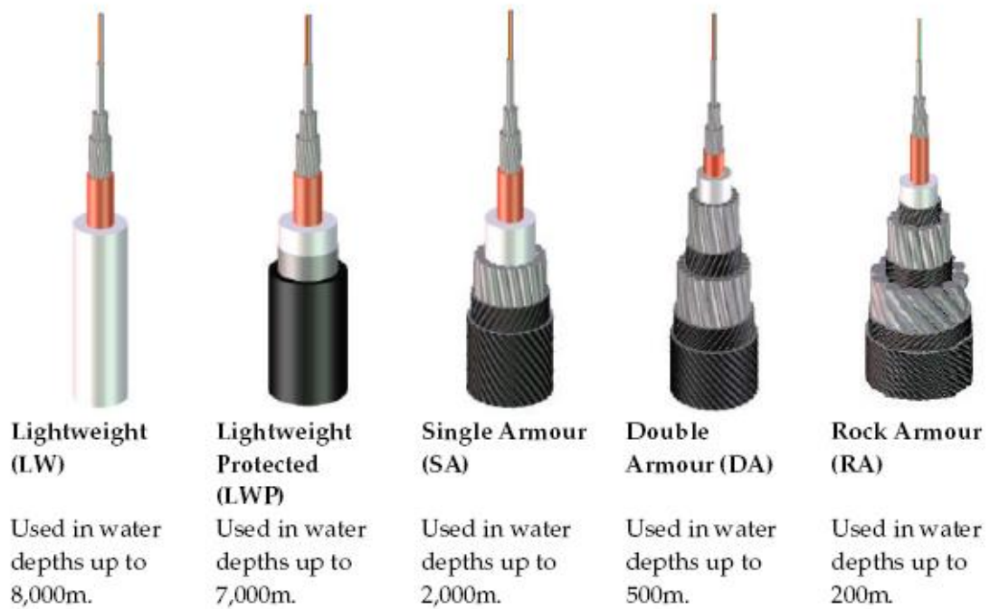
Plate 2 Cable armoring and operational depths
