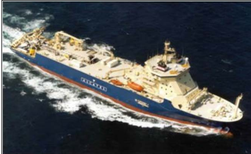
Figure 2 Typical Cable Laying Ship
