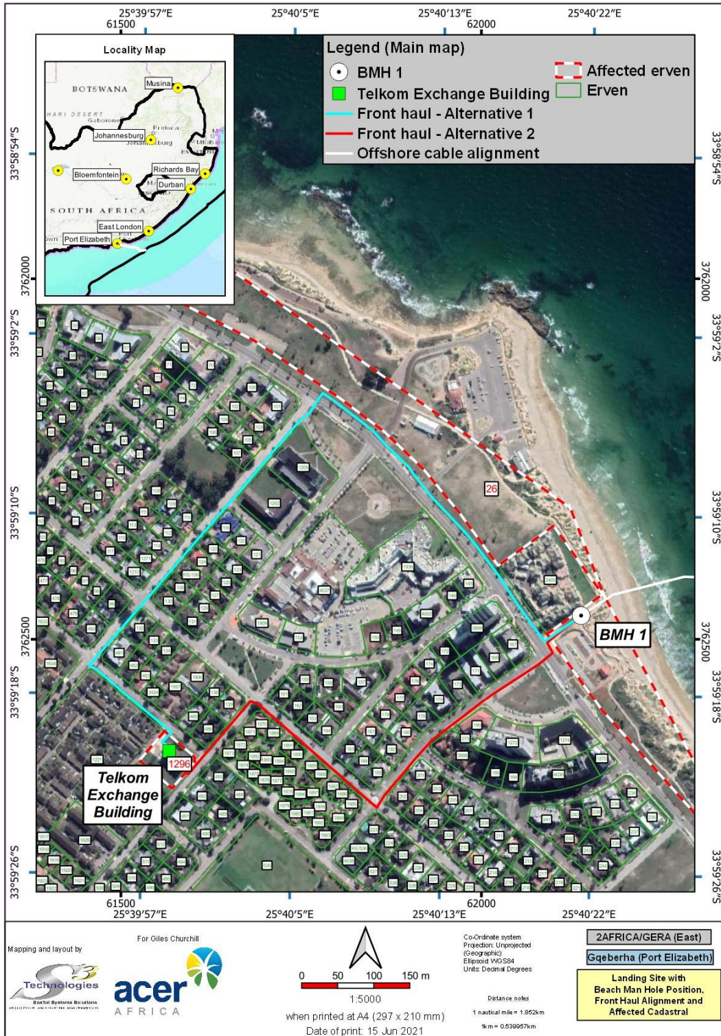
Figure 8 Image showing the selected landing site, BMH and selected front haul alignment (blue line) to CLS at the Telkom Exchange Building
