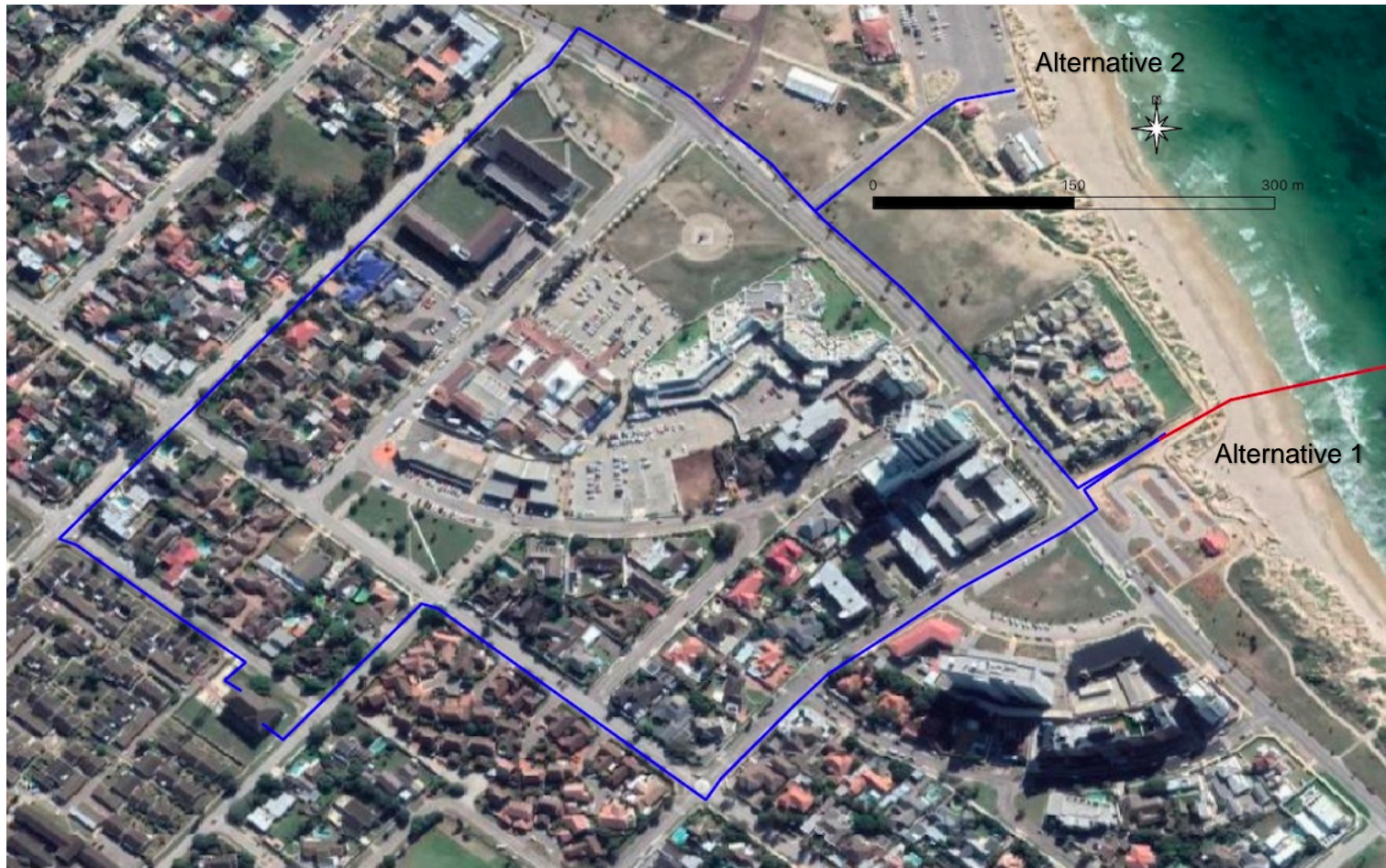
Figure 3: Proposed terrestrial cable route options (blue lines) between the two possible landfall and BMH sites on Pollock Beach and the Cable Landing Station on the corner of Skegness and Bognor Streets, Summerstrand. The marine cable (red line) terminates at the BMH. Alternative 1 is the preferred BMH site (Source: Google Earth).
