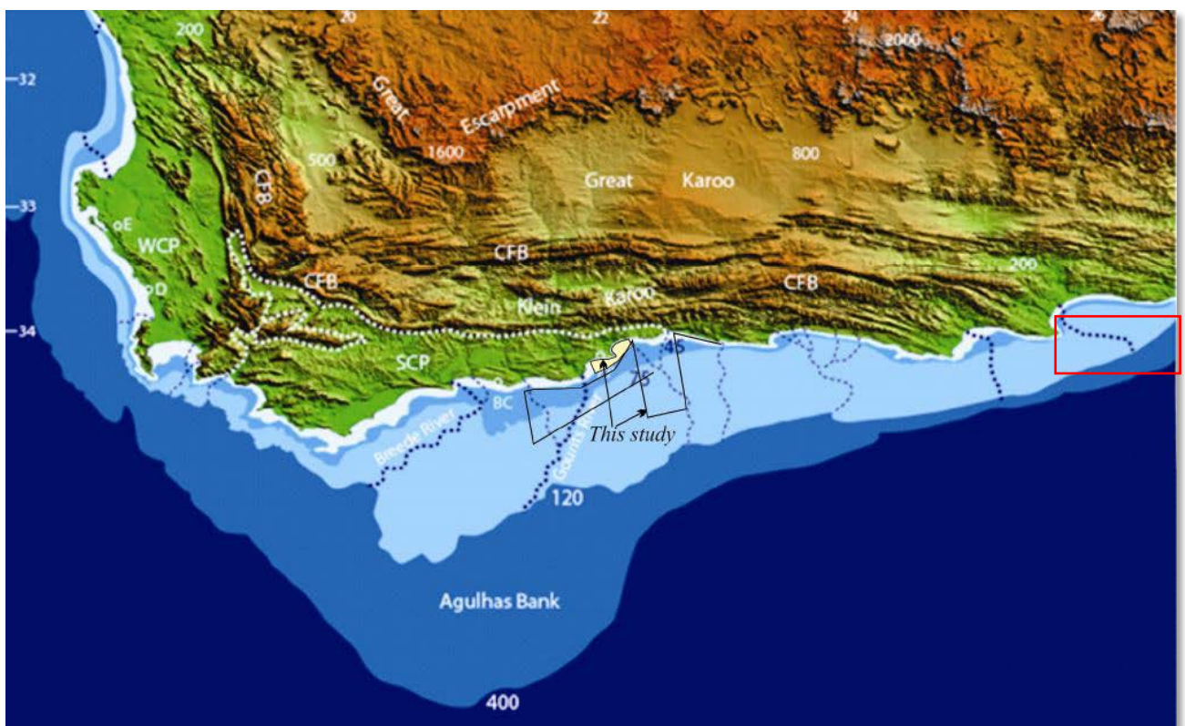
Figure 6: The south coast continental shelf showing the water depths of 45, 75, 120 and 400 m. The 2AFRICA/GERA (East) branch cable to Port Elizabeth will be installed in the area highlighted in red on the right of the image (Source: Compton, 2011 from Cawthra, 2014).
