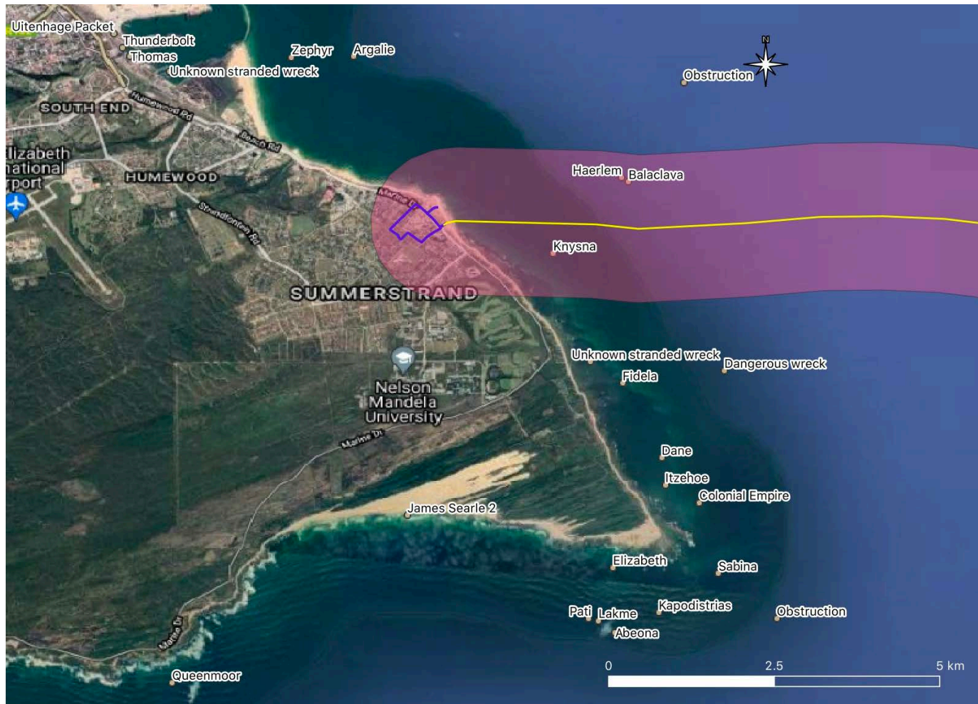
Figure 12: Proposed alignment of the 2AFRICA/GERA (East) cable system within Algoa Bay. The maritime assessment study area (a 1 km buffer on either side of the route) is shown, as are the recorded wrecks in the vicinity, both to the north around the old anchorage, and to the south around Cape Recife (Source: Google Earth).
