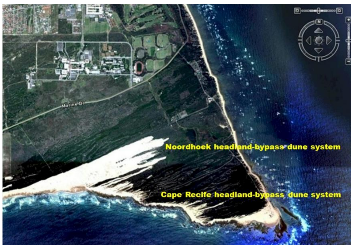
Figure 10 Noordhoek headland-bypass dune system which has been blocked off by the development of a sewage works and the smaller Cape Recife headland-bypass dune system near Cape Recife point.
