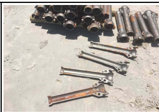
Plate 10 Articulated pipe sections which will be installed around the cable in shallow water to offer additional protection.
