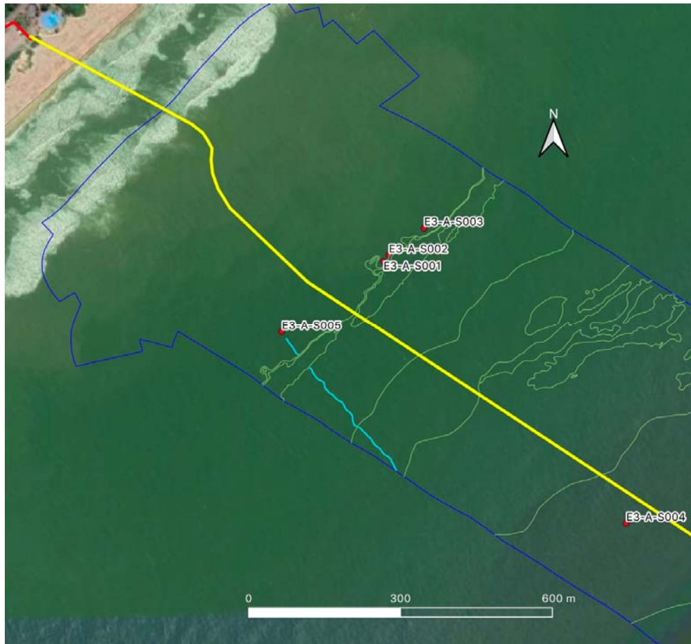
Figure 14: SSS contacts (red dots) including the anchor block (E3-A-S005) and possible associated linear contact (anchor chain?) (light blue) (Source: Fugro Marine Germany survey data).
