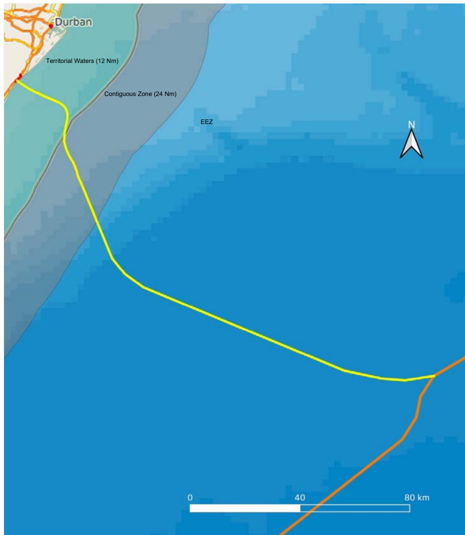
Figure 2: Alignment of 2AFRICA/GERA Amanzimtoti branch line (yellow) from main cable route (orange) to the landfall (Google Earth).
