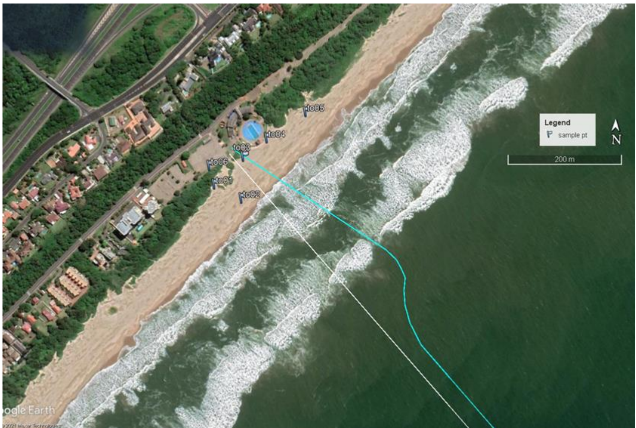
Figure 5. Image showing sample points in relation to proposed cable landing point, showing possible cable routes .
