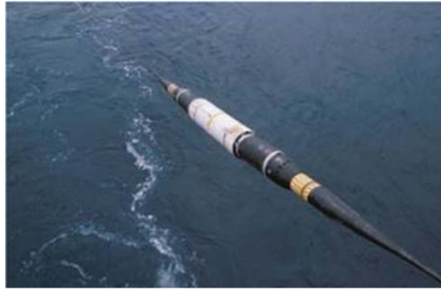
Plate 3 Example of a repeater
