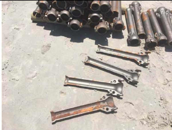
Plate 9 Articulated pipe sections which are installed around the cable in shallow water to offer additional protection.
