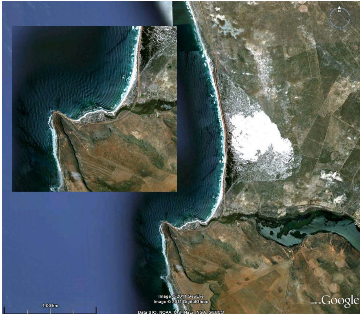
Figure 20 Log spiral bay development at Elands Bay showing wave refraction around the headland (Source: Umvoto Africa, 2011)
