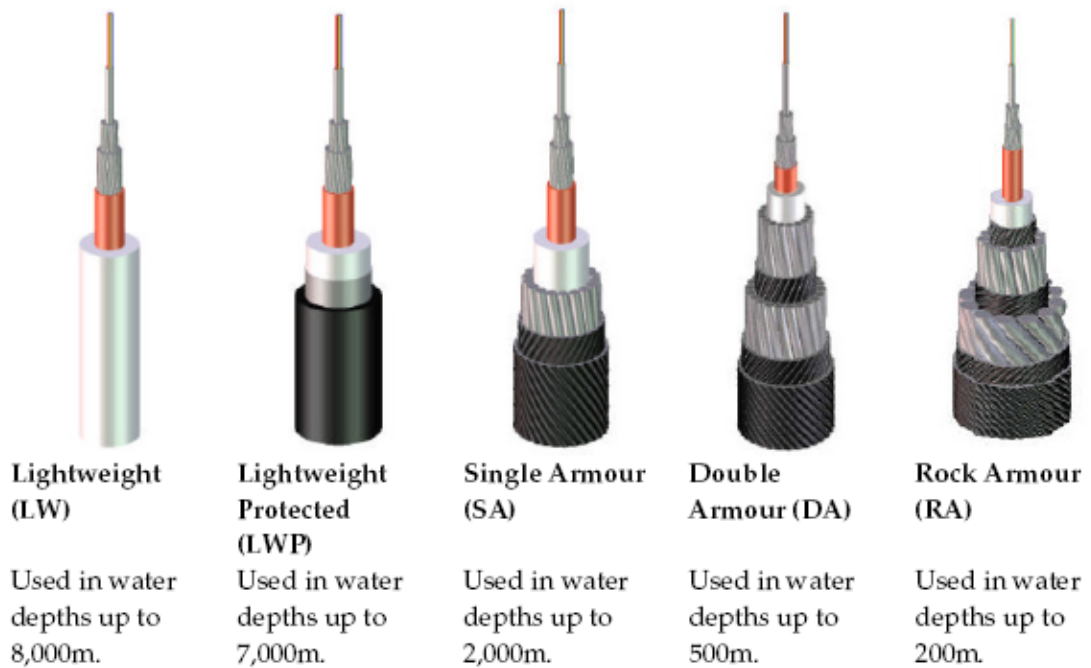
Plate 2 Cable armouring and operational depths
