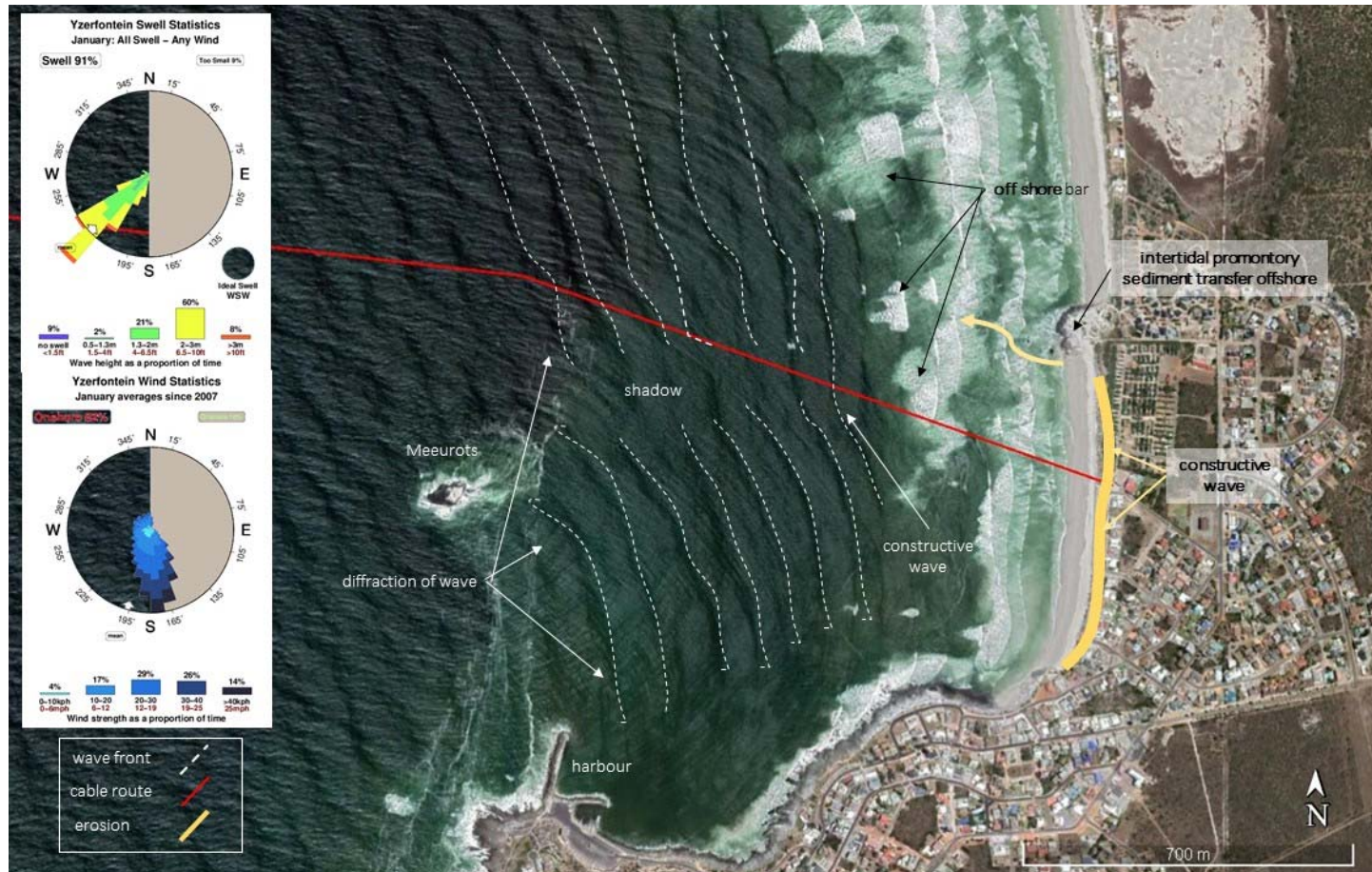
Figure 37 Aerial photograph showing features and coastal dynamics at site of cable landing, Yzerfontein
