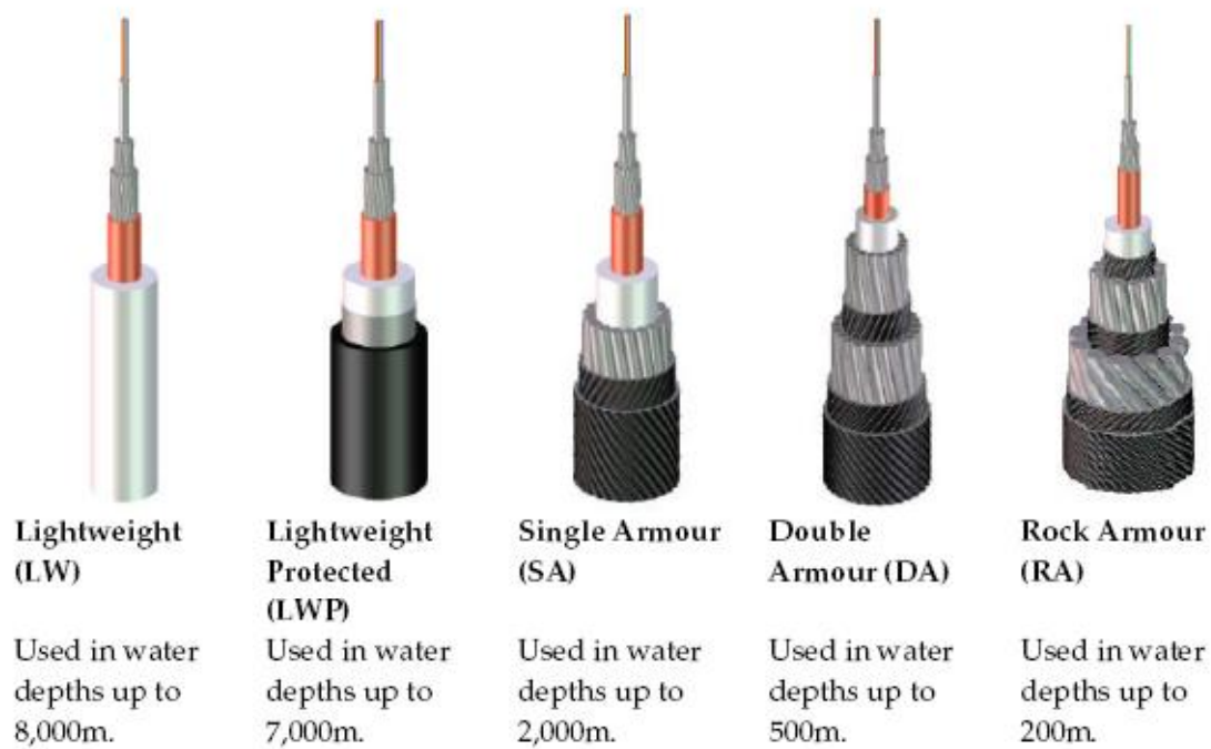
Plate 2 Cable armoring and operational depths
