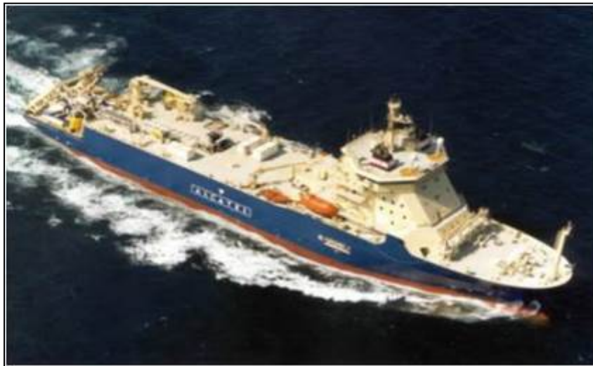
Figure 2 Typical Cable Laying Ship
