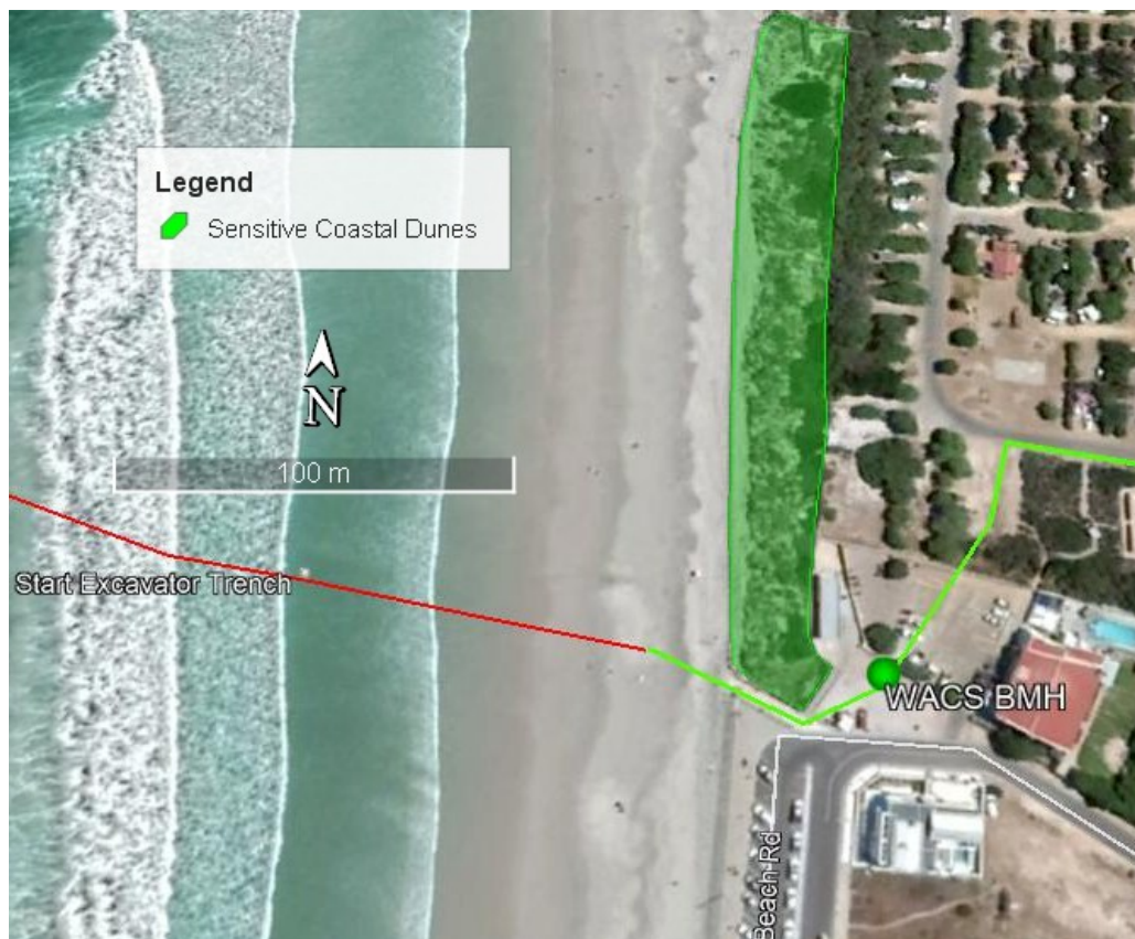
Figure 8 Alternative 1 - preferred landing site and position of the WACS Cable System Beach Man Hole (Source Google Earth 2020)
