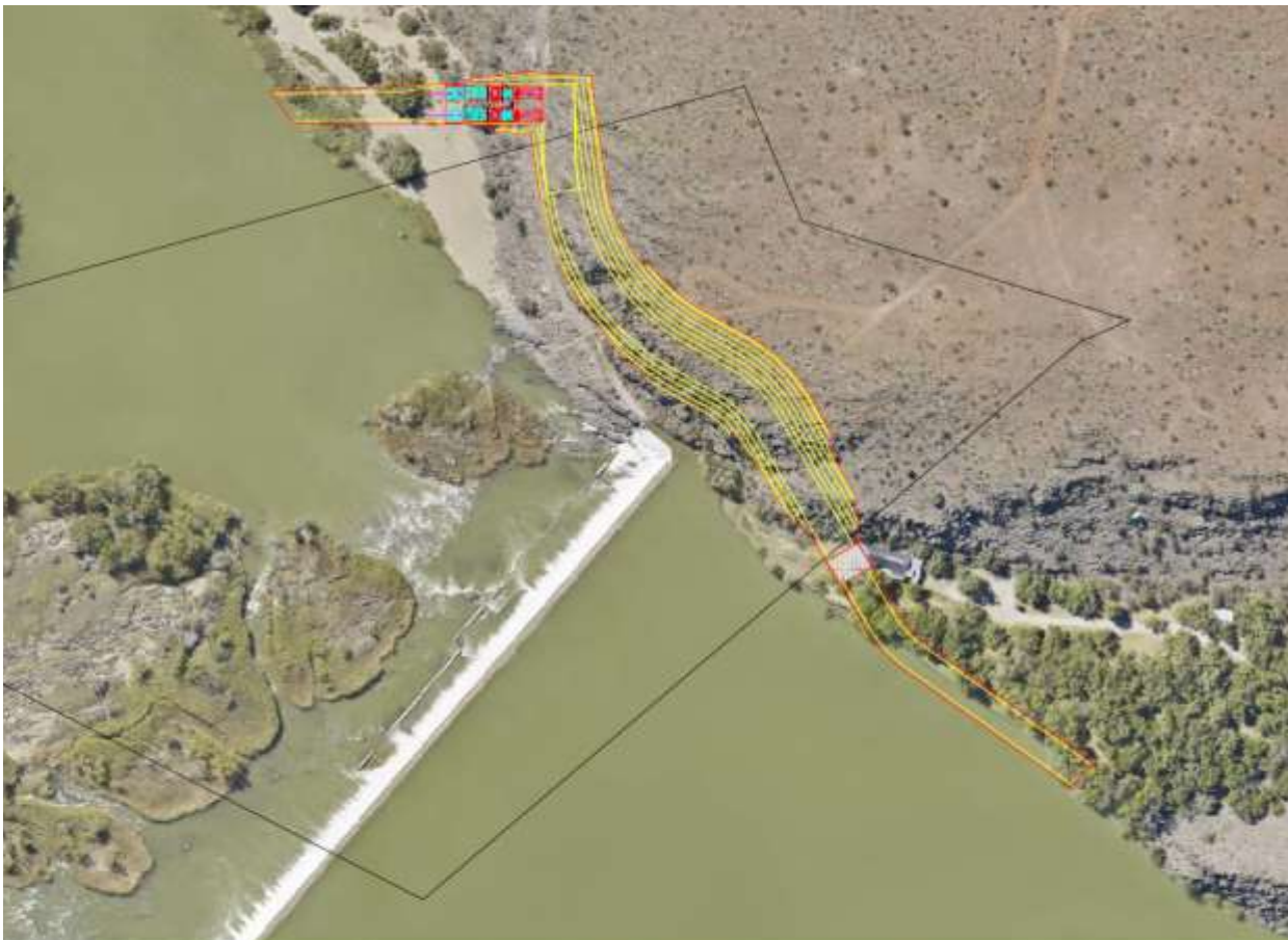
Figure3. Sketch of the layout of the Boegoeberg Hydropower Facility, with the off-take weir and inlet structure situated just upstream of the weir (bottom right in picture), and the head-pond, power-house and tail race just downstream (top left).
