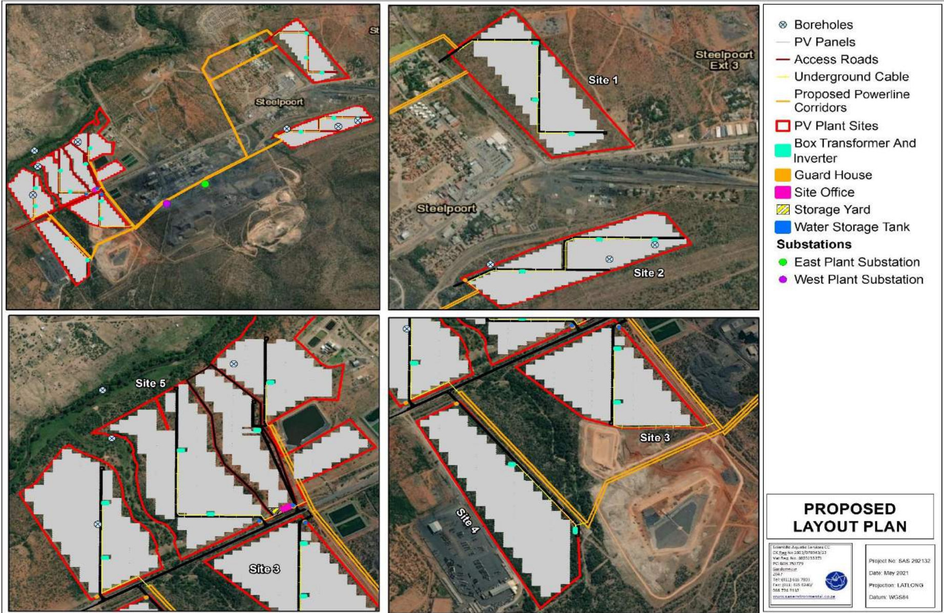
Figure 3: Proposed layout of the PV Plant Sites and the associated powerlines and their alternatives.
