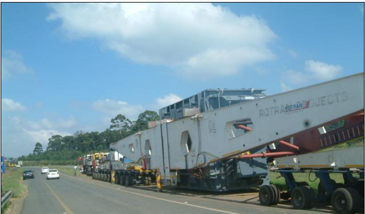
Plate 6: Large transformers being transported to the substation site
