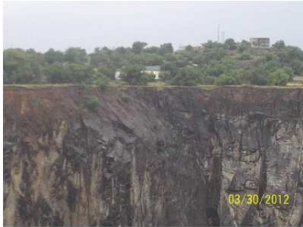
Figure 4-12 : Flatter joint dip angles in dolerite
