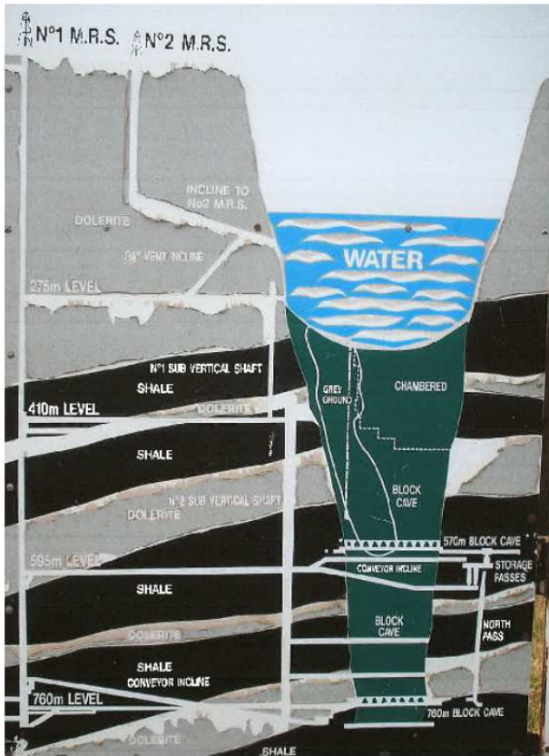
Figure 4-3 : Coloured cross-section of open pit
