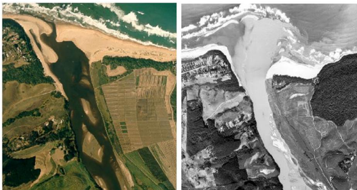
4 5 Figure 3: Thukela Estuary under low flow conditions with a stable channel meandering between sand banks (left) and 6 the Thukela Estuary under resetting flood conditions with high volumes of sediment being eroded from the system 7 (right).
