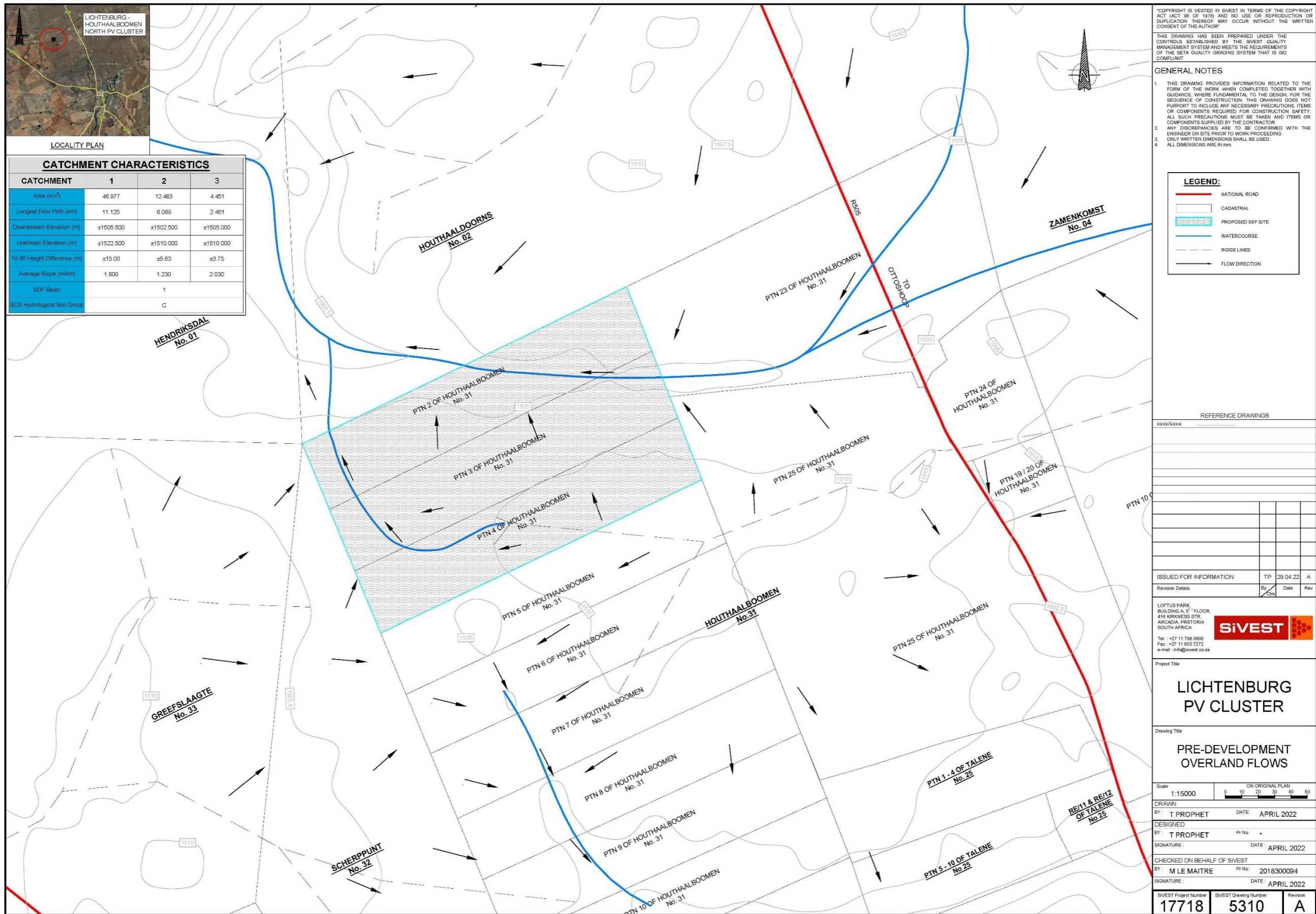
Figure 11:3 Euphorbia PV Development Area– Pre-Development Overland Flow
