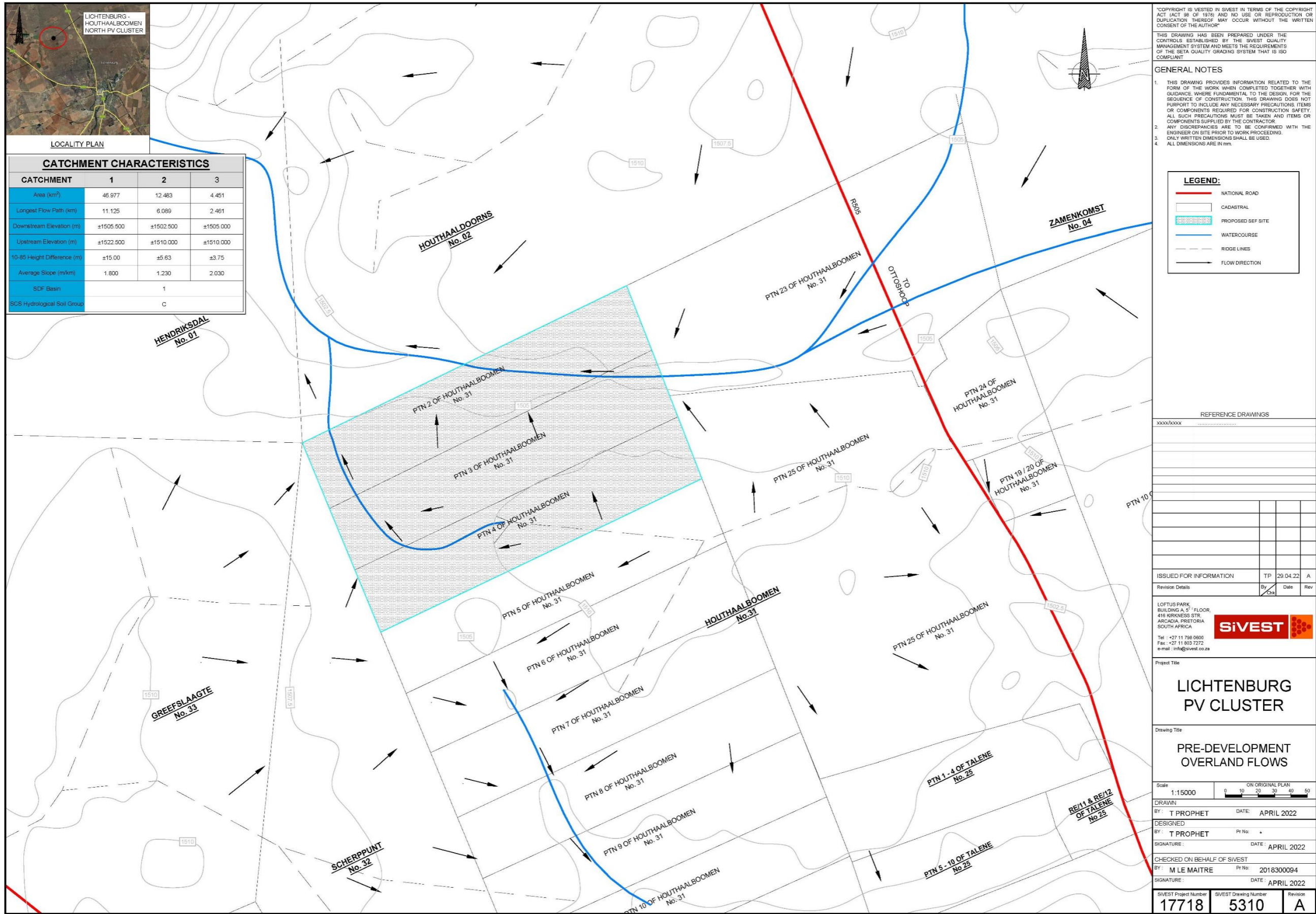
Figure 11:3 Hillardia PV Development Area- Pre-Development Overland Flow
