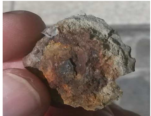
Photo 4.4 & 4.5: Skimming grout covering fixing lugs is popping off due to corrosion at the fixing lug.
