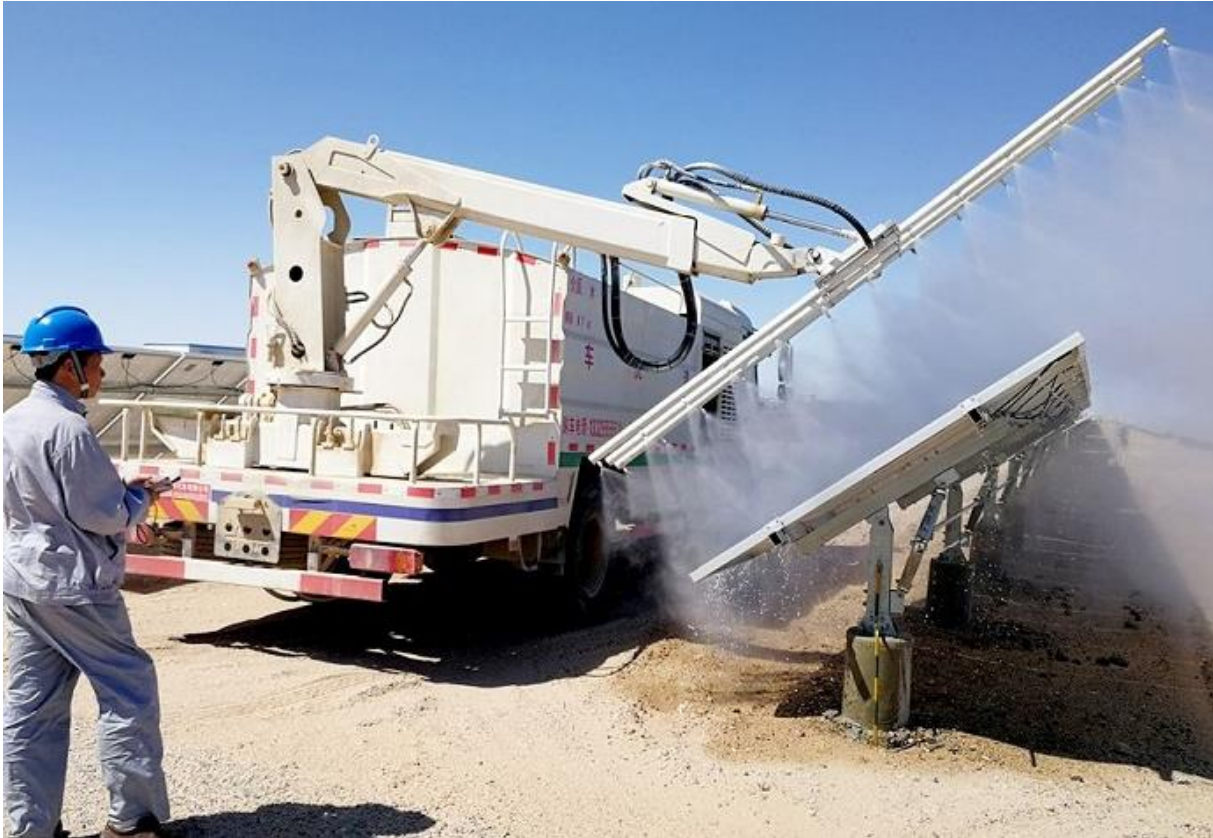
Figure 6-1: Mechanical Solar panel cleaning system
