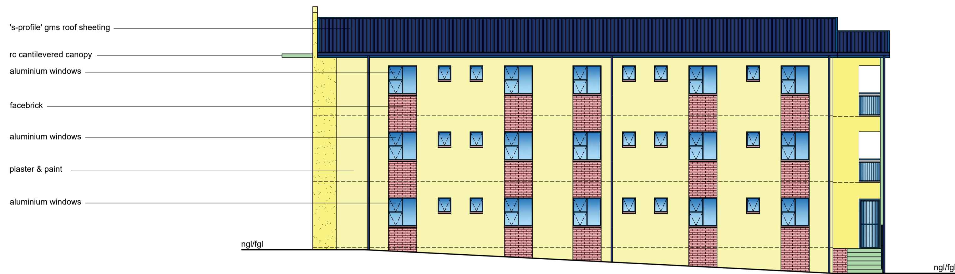
SOUTH WEST ELEVATION
