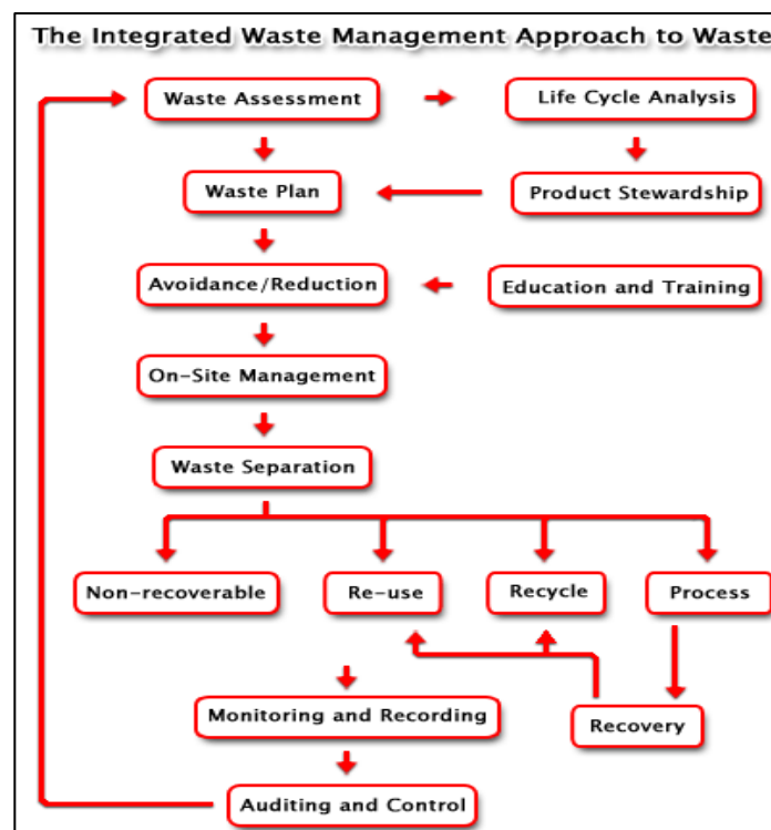
Figure 1: Integrated Waste Management Flow Diagram
