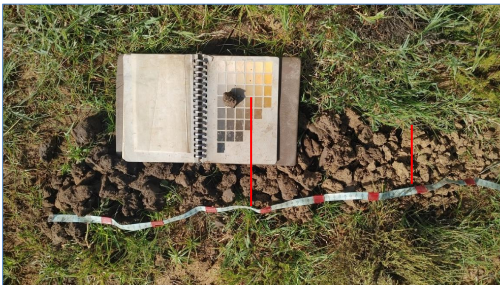
Figure 9: Image illustrating from left to right, the Melanic A horizon, followed by the G 1 and G2 horizons of the wetland soils
