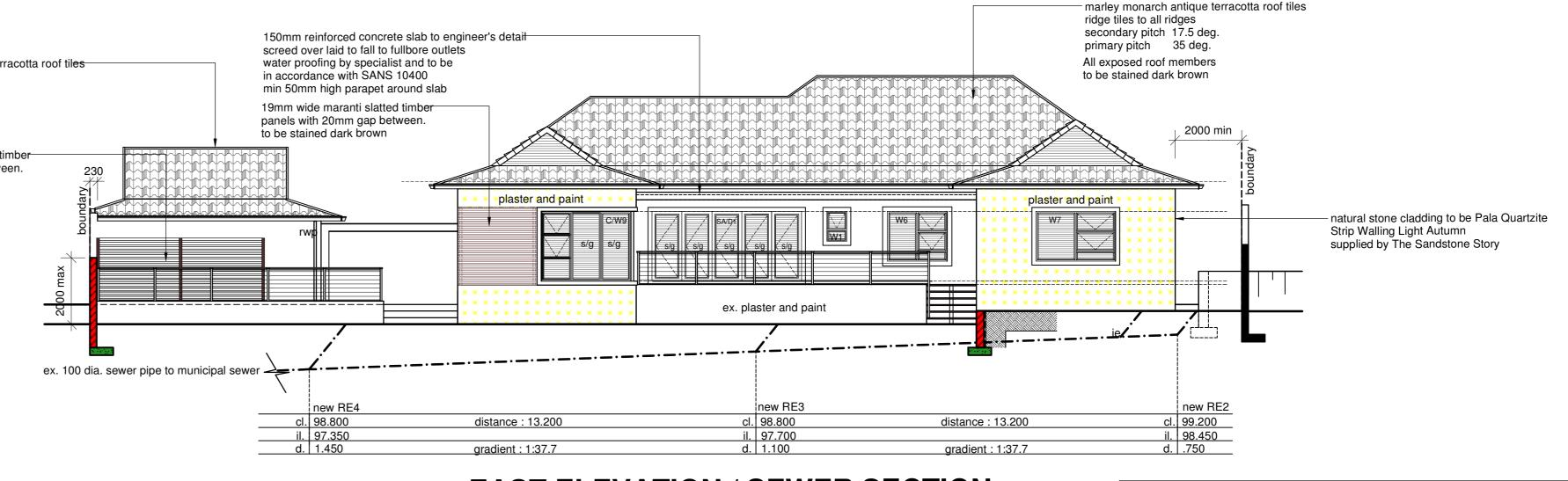
EAST ELEVATION / SEWER SECTION SCALE: 1:100
