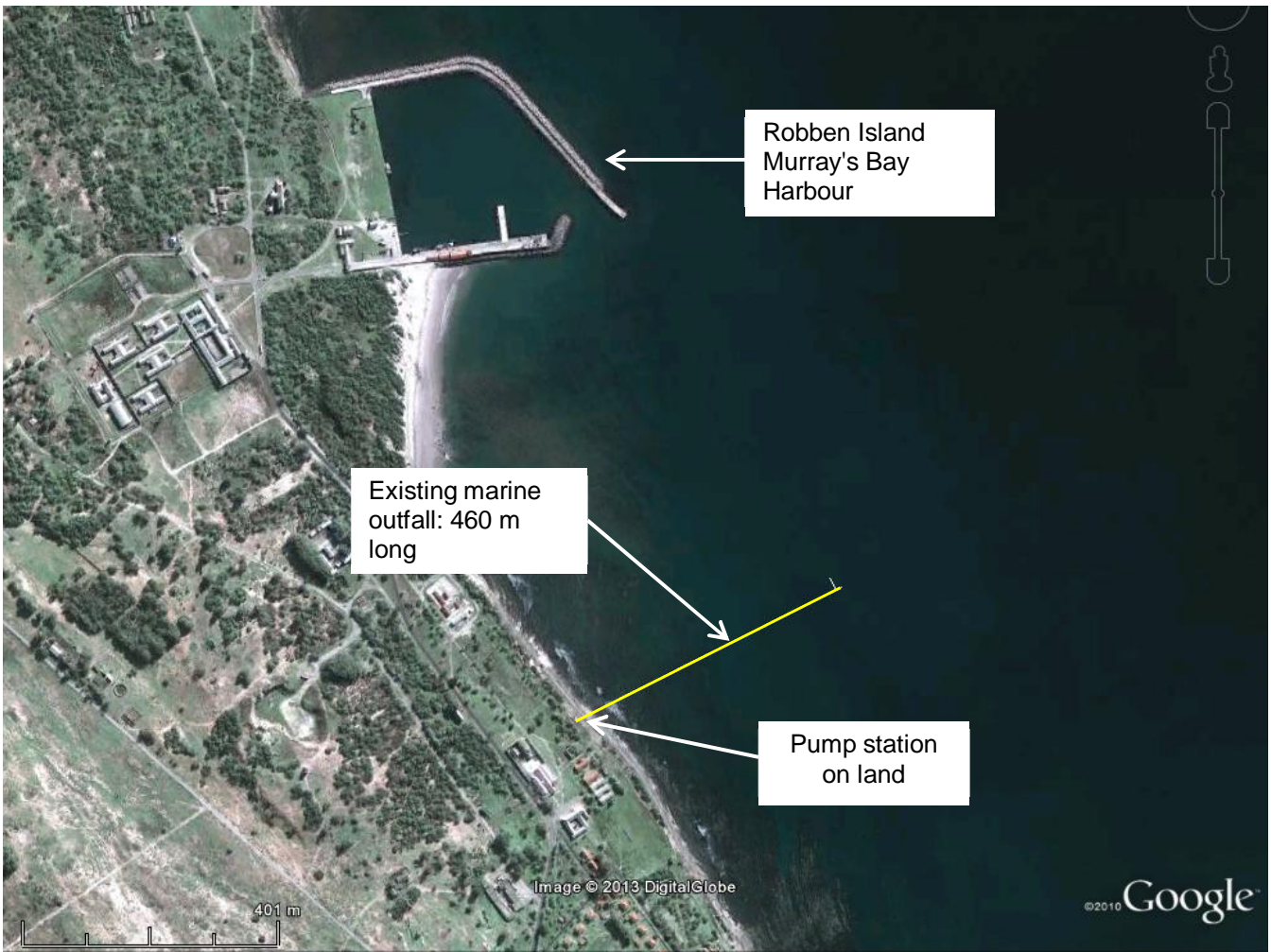
Figure 1.1: Location of existing marine outfall
