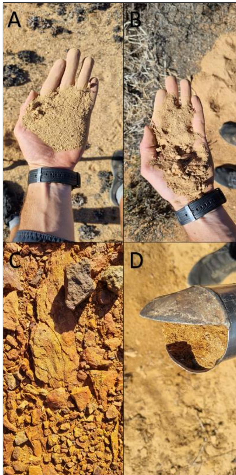
Figure 1. Soils found within the proposed project area; A) Alluvial material on top of a hard rock; B) sandy chromic orthic topsoil that is underlain by saprolithic horizon; C) Bare rock; and D) Neocarbonate horizon with the presence of sporadic carbonates.
