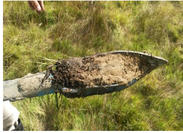
Figure 16: Soil sample collected in the floodplain wetland with an orthic G Horizon indicating clear signs of wetness.
