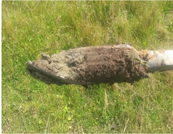
Figure 9: Sample collected in the floodplain wetland with an orthic A topsoil with an E horizon indicating clear signs of wetness.
