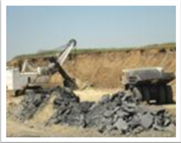
i) Truck and shovel methods of overburden material
