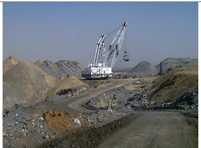
f) One of the two Draglines operated at Isibonelo Colliery
