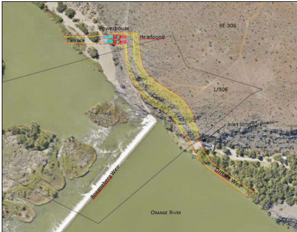
Fig. 2. Layout of the main infrastructural components of the proposed Boegoeberg hydropower station on the River Orange River (Image abstracted from the Final Scoping Report by Aurecon 2013).
